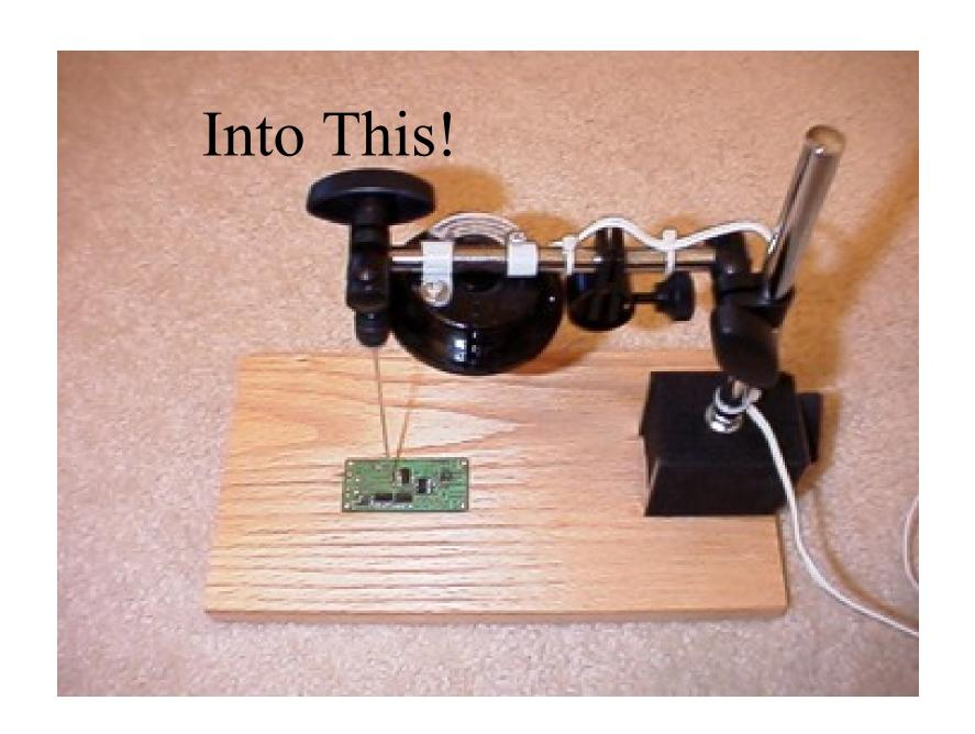
• Here's a handy tool for soldering SMT parts onto a printed circuit board. It holds SMT parts securely to the board while soldering. In addition, the weight of the tool is such that you will no longer have to chase your pc board around the work bench while you are soldering.
